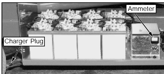
Figure 6: Power Module, Chassis Right Side
